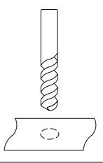
4. USING A 35mm HOLE SAW WITH A DIAMOND TIPPED CUTTER, POSITION THE GUIDING DRILL BIT INTO THE PILOT HOLE.
