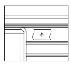
3. DRILL A PILOT HOLE THROUGH THE CENTRE OF THE MARK. THIS WILL HELP YOU WITH THE POSITIONING THE 35mm CUTTER.
