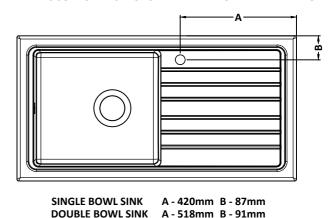
2. USE MASKING TAPE TO PROTECT THE SINK SURFACE AND MARK YOUR DESIRED POSITION WITH A PENCIL OR MARKER.
